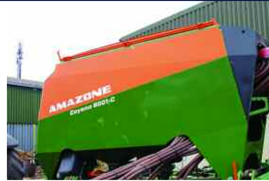
C specification machines have a 60:40 split 4000-litre hopper, and Alan has made use of this to place some TSP at drilling where possible.
