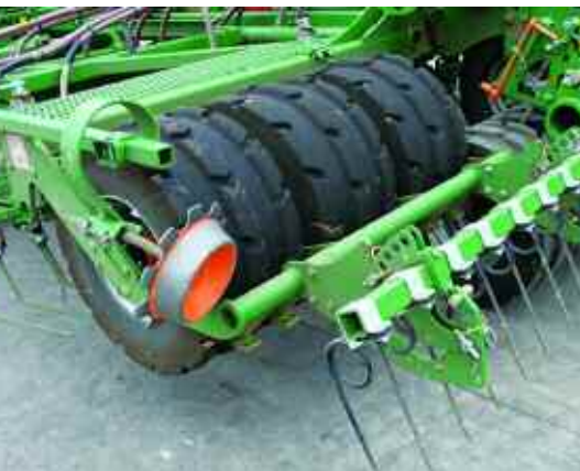
Tine coulters are followed by angled sweep tines, 800mm rubber press wheels and covering tines.
