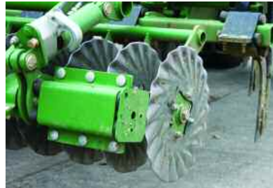
Leading wavy-edged discs each cut a path for the tine coulters behind, and create a small amount of tillth.
