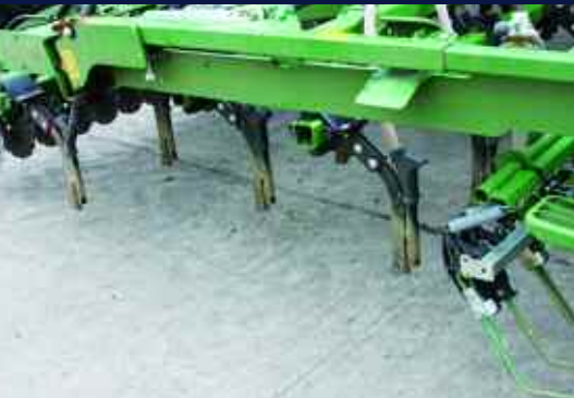
The 36 narrow coulters are arranged over three rows, and spaced well for good trash flow.
