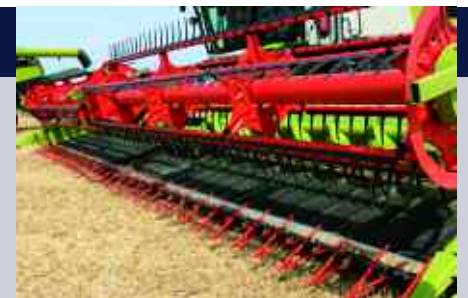
The Convio Flex has a flexible knife and cutterbar.
