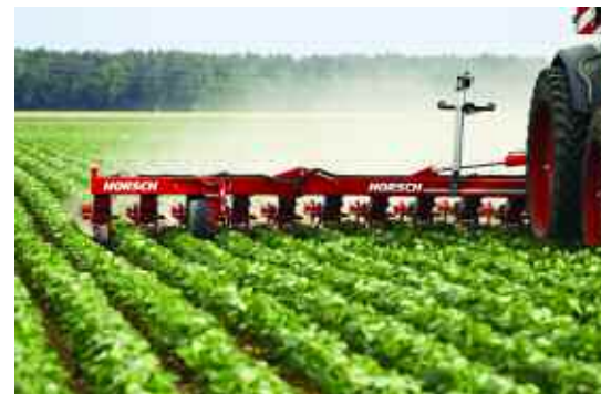
A variable frame design allows the Transformer VF to work in row crops spaced at widths from minimum of 25cm up to 90cm.
