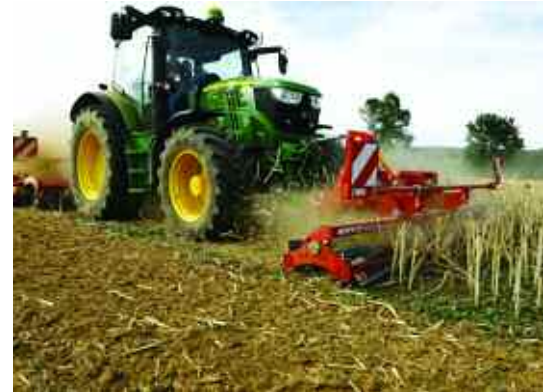
The Cultro TC stubble processor is available as a 3m front or rear-mounted model, or in 12m trailed format.
