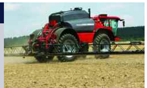
There are two models in the new Horsch Leeb self-propelled range, with 6,000- and 8,000-litre tank capacities.
