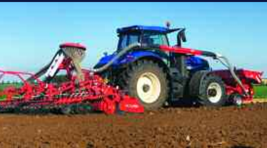
With a 6m working width the BTFR 6030 includes the Kuhn Seedflex coulters seeding unit.
