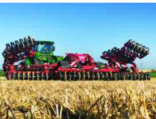
The folding mounted Prolander 100 R range has a low power requirement of 25-35hp/m.
