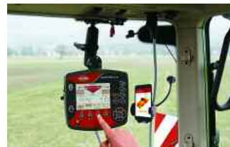
EasyMaps displays application maps in real time and can indicate the required application rate and variation percentage.
