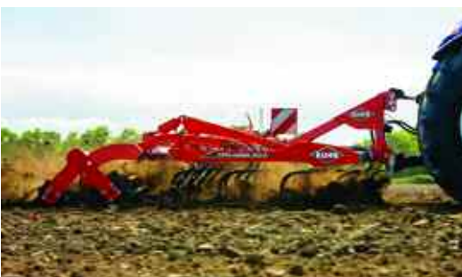
The folding mounted Prolander 100 R range has a low power requirement of 25-35hp/m.
