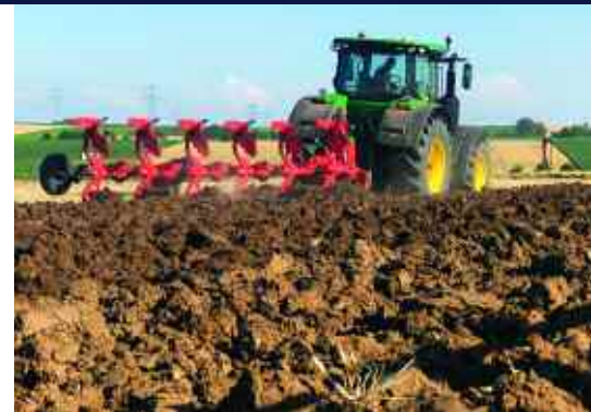
The Line element of Smart Ploughing adjusts the working width of the plough using GPS, and can take account of field irregularities.
