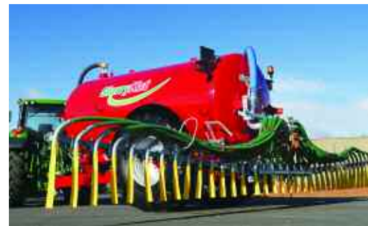
The 12m vertical folding dribble bar can be tanker-mounted or used on an umbilical system.
