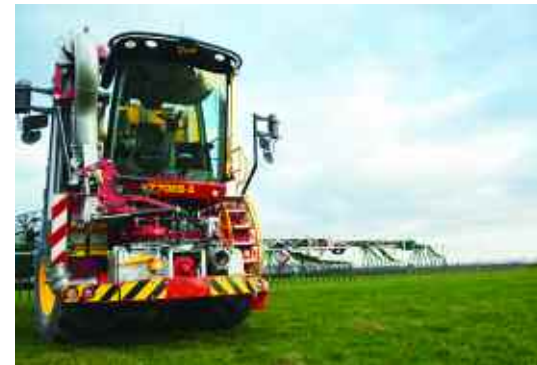
In the guts of the new Vredo VT7028 spreader is the Deutz 16-litre V8 engine with 687hp.
