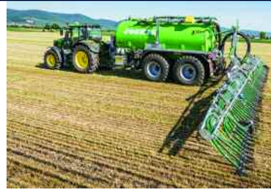
The John Deere Manure Sensing allows users to apply N, P and K more precisely.
