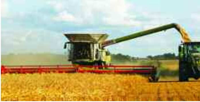
Although there have been some pre-production teething troubles with it, the new unloading system is praised for the rate at which it empties the 16,000-litre tank.
