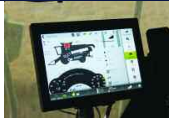
The new CEBIS screen eases the task of finding the best settings for a crop, with a tap on the touchscreen bringing up everything needed.
