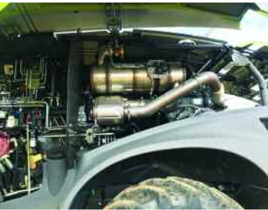
Instead of using the old-style V configuration, the 970 model now has a new straight 6 big block engine.
