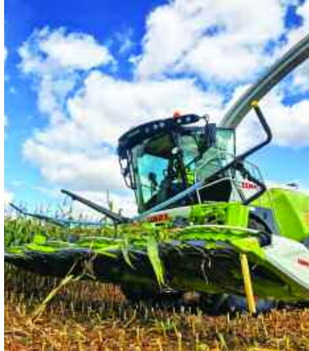
Claas has introduced a 42-blade option, and the main reason for this is for biogas throughput.
