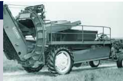
The first self-propelled Grimme machine combined the front part of a Deutz tractor with a single-row Europa Standard potato harvester.
