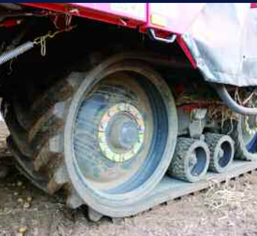
The 900mm Terra Trac unit has been moved a few cm, making quite a difference to the turning circle and stability.
