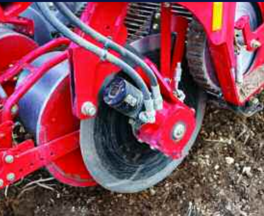
A powered drive to the discs at the front improves crop flow and ensures no blockages.
