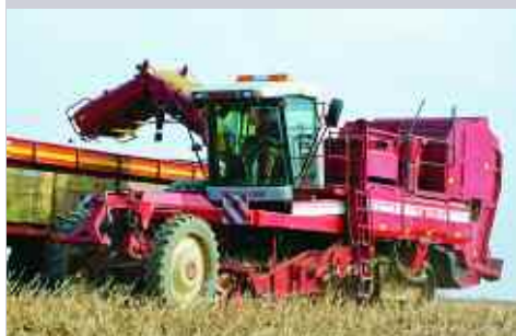
The two-row SF1700 GBS, built until 2009, was specifically built for the UK grower and included a cart elevator.
