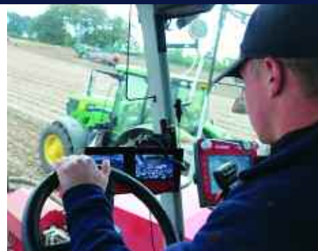
Visual Protect automatically switches the display to the relevant part of the machine if Oli makes an adjustment on the move.
