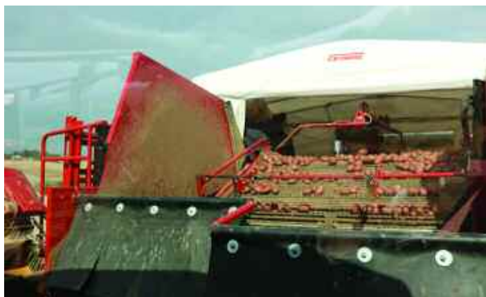
The picking table passes into a 2t buffer bunker, so there's no waiting for the trailer to line up.
