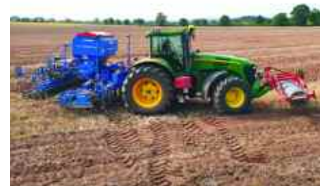
A Lemken Solitair combines six operations into one and does much of the work on the Solari's farm.
