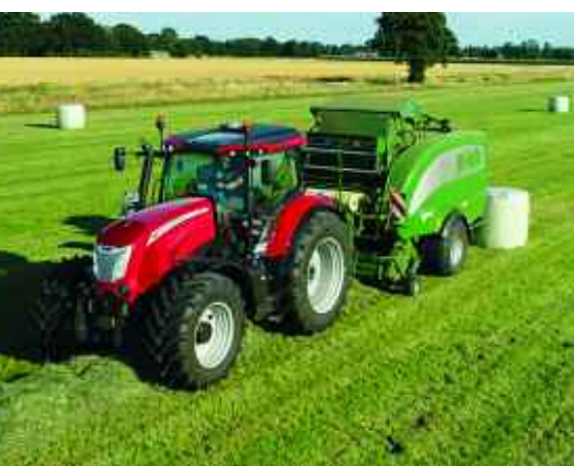
Equipped with a six-cylinder, 24-valve 6.7-litre engine, the McCormick X7.624 delivers a maximum torque of 983 Nm at 1400 rpm.
