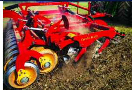
Designed for conserving moisture in the seedbed, Väderstad’s cultivator has the ability to work at ultra-shallow depths of only 3cm.
