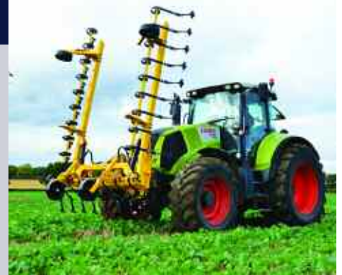
Claydon's TerraBlade Inter-row has been designed to help eliminate weeds alongside herbicides in both conventional and organic arable systems.
