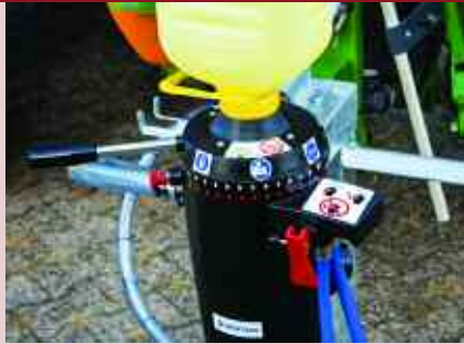
Easyconnect’s screw cap fits to a coupler, which transfers the product directly into the spray tank and rinses the container.
