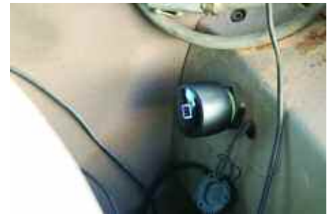
The FieldView Drive plugs into a tractor or combine controller area network (CAN) diagnostic port.
