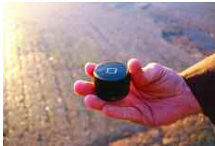
The FieldView Drive plugs into a tractor or combine controller area network (CAN) diagnostic port.
