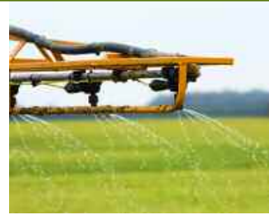
Operating nozzles within the correct pressure range to produce the recommended droplet size will mitigate the risk of scorch occurring.
