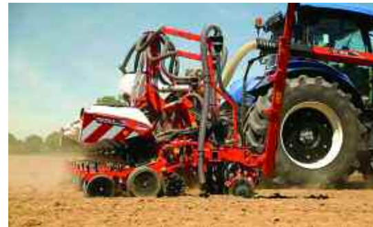
Row-by-row seed rate variation is now possible in electrically driven models within Kuhn’s Maxima 3 precision drill range.
