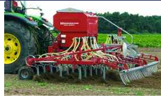
The Kongskilde Vibro Seeder combines a spring tine cultivator with a pneumatic seed drill.
