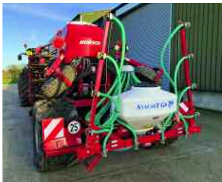
The powerful hydraulic fan provides air to deliver Avadex at widths of up to 12m.
