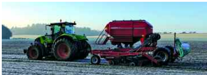
The Avacast GR 200 is a granular applicator specifically designed for applying Avadex micro-granules.
