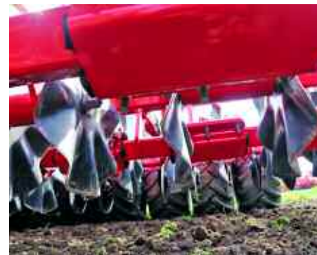
There are two rows of 510mm diameter wave discs on the Terrasem, which each work a 45mm-wide strip to a depth of just 10-15mm.
