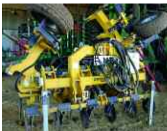
Fitted in front of the drill with low disturbance legs, the Grange toolbar puts air into the soil and allows one-pass establishment.
