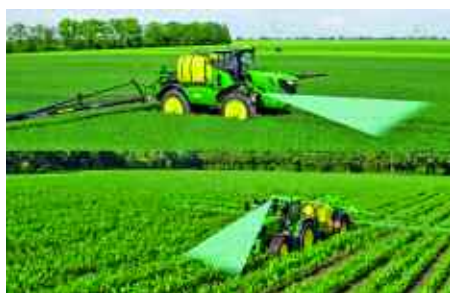
To help improve precision within self-propelled sprayers, John Deere launched its AutoTrac Vision system for self-propelled sprayer models.
