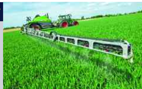
Fendt's trailed Rogator 300 recently received an update, increasing boom width to up to 36m.
