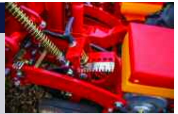
Seed depth is adjusted via an excenter-lever.
