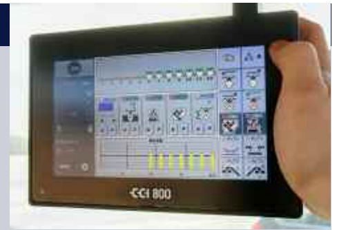
The CCI 800 has a 200mm multitouch screen.
