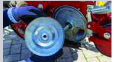
The seed plates come with six holes as standard, while an eight-hole plate is also available.
