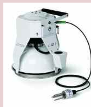
A soil gas flux analyser was used which is a portable instrument with a bell-shaped chamber that can detect six different gases simultaneously.
