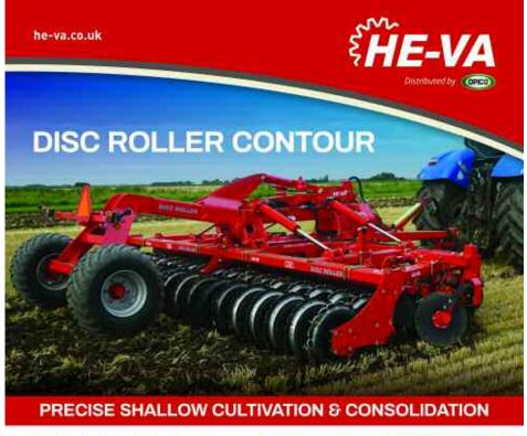
Precise depth control and contour following gives uniform soil movement across the full operational width - vital if employing reduced tillage or creating stale seedbeds for blackgrass control.
