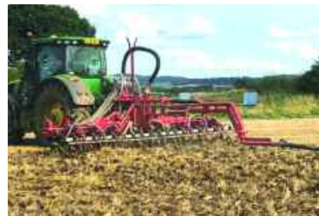
The Evers slurry injector, band-applies 50kgN/ha to the OSR crop, giving it a valuable kick start.
