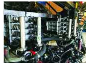
*Perhaps one of the most interesting pieces of tech in the demo ring was the MagGrow system — a retrofitted sprayer attachment that magnetises fluid to improve droplet size.*
