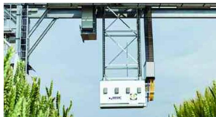
*Rothamsted used the event to showcase its Field Scanalyzer system — which is claimed to be the world’s first field crop analytics facility.*
