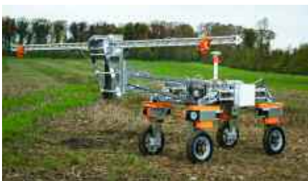
Currently carrying out pre-commercial trials, the two high-detail cameras mounted on SuperTom's 4m boom are being replaced with six lower-detail devices.
