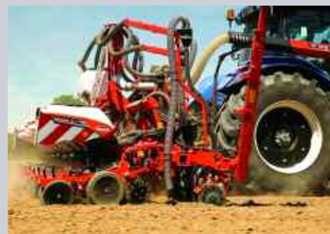
At the start of the year, Kuhn also announced that row by row seed rate variation was now possible in electrically driven models of the Maxima 3 precision drill range.
