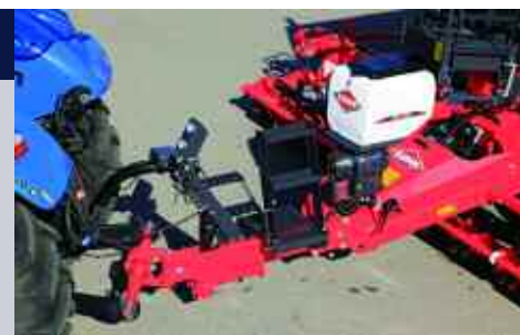
Kuhn has introduced a range of supplementary seeders to facilitate progressive practices such as companion cropping or to apply fertilisers, granular herbicides or slug pellets while drilling.
