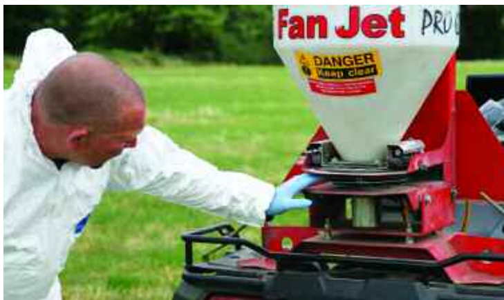
Every brand of slug pellet has different ballistic properties and application equipment should be recalibrated for each type.
