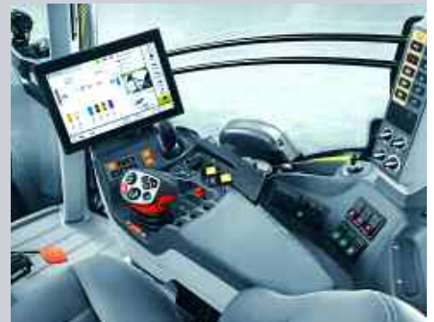
As with the Arion, all CEBIS Touch-equipped machines now come with ISOBUS UT as standard, allowing it to be used as a universal implement control terminal.
