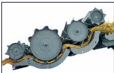
Central to the all-new threshing system is a 755mm-diameter drum, coming in at a rather impressive 26% larger than the 600mm drum on the Lexion 600 range.
