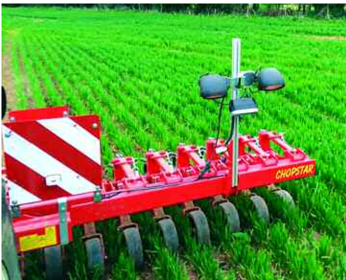
Glebe farm has been using New Holland’s IntelliSteer system on an interrow hoe to help improve weed control.
