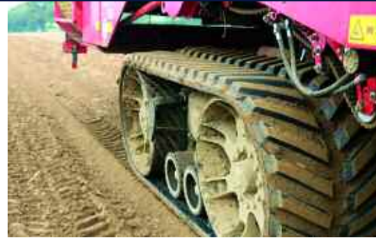
The Varitron's a larger machine, but the weight distribution on its Terra tracs is much better than a tractor and trailed harvester.
