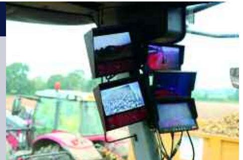
Visual Protect prioritises which of the machine's eight cameras feed the two displays in the cab, while three more have been added to increase visibility.
