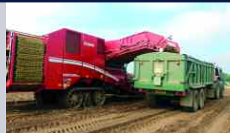
The unloading elevator itself has a 600mm extension and is set in three sections.
