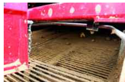
There's a gentle shallow intake over the webs with less roll back and a massive sieving area.
