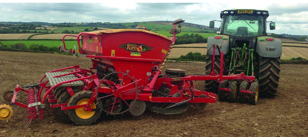
The Väderstad Rapid drill can cover up to 40ha of OSR per day but has been the Achilles heel in the system for the past couple of years.
