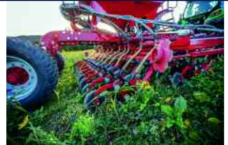
The Avatar boasts a stable depth control wheel for precise positioning of the coulters in changing or difficult soil conditions.
