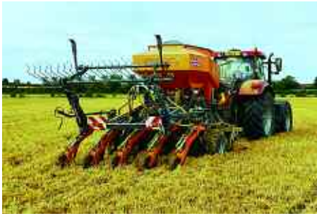
The Mzuri focus at Springfield Farms is on creating a suitable micro-climate for young seedlings from the start by drilling into 200-250mm of standing straw.
