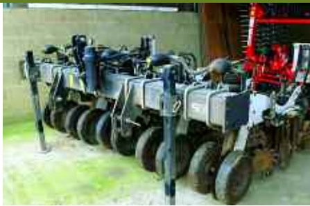
A Sly Stripcat (left) is used to pull cultivated strips, or berms, through the cover crop into which the maize is planted a month to six weeks later.
