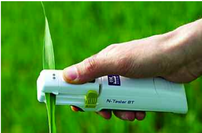
The N-Tester BT connects to a smartphone and needs at least 30 readings on the last leaf to fully emerge to give an accurate value of chlorophyll content.
