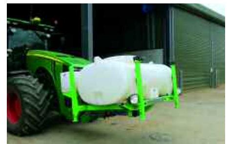
The “gloopy” biological mixture is pumped from the front-mounted tank directly to the cross-shaped seed coulters on the drill.
