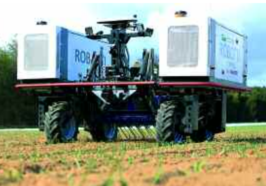
Field obstacles such as telegraph poles or trees are logged at the programming stage of the Robotti.
