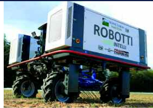
The model at Home Farm has two Kubota 75hp diesel or bio-fuel engines.
