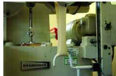
The tensile tester measures the properties of the functional protein of a potential bread-making wheat variety.
