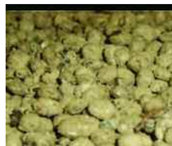
The OMF was produced by drying sewage sludge cake in a tumble dryer from 25% dry solids to 80-85%.
