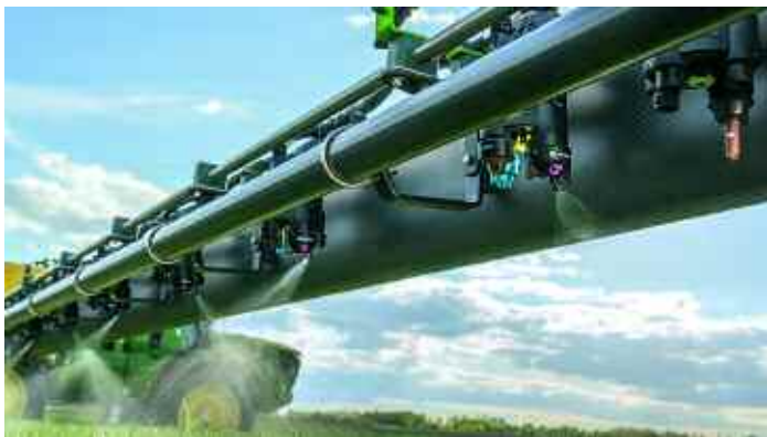
ExactApply technology uses pulse width modulation to spray at a constant pressure and enables growers to control each individual nozzle, independently to the pressure.
