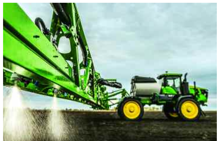
While not available in Europe, Deere's See & Spray technology can identify weeds and apply a herbicide at specific locations across the field, using AI and high-speed cameras.
