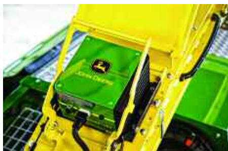
With the John Deere HarvestLab sensor, the precise nutrient content of manure can be accurately measured.
