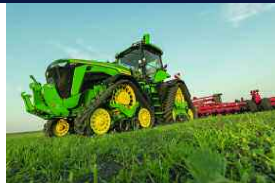
The new John Deere four-track 8RX has a huge footprint of 4.6m 2 , so the contact surface pressure is very low at only 0.4kg/cm 2 .
