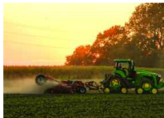
The 8RX's larger footprint also means less track depth, which reduces compaction in the deeper soil layers and reduces roll resistance.
