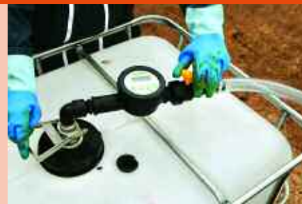
The new FasTran 850 closed transfer system for liquid MH will save half an hour per sprayer fill-up, reduce operator exposure and eliminate waste packaging.
