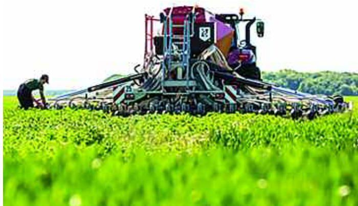
The Novag T-Force range are true no-till, ultra-low disturbance disc drills.
