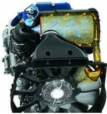
The new 900 and 1000 Vario series feature a new self-cleaning air filter.
