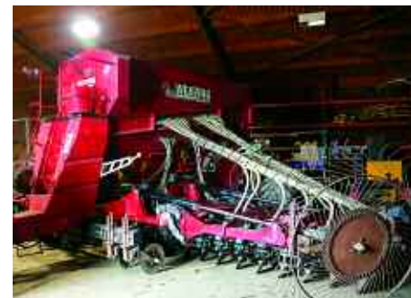
A hay rake tine wheel has been attached at each end of the Weaving GD8000T drill.
