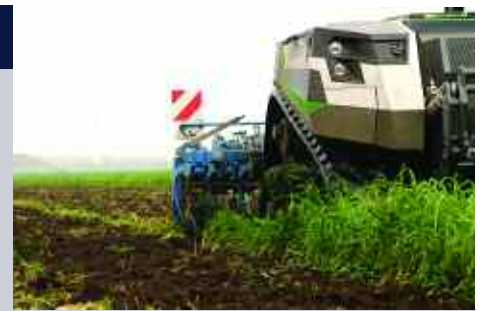
The AgBot Ecosystem is a digital path planning, autonomous task performing and automatic data collection robot, controlled with just a couple of clicks.
