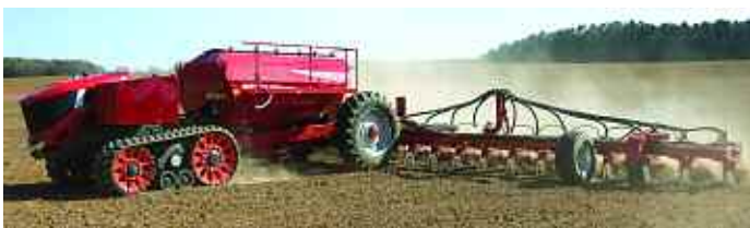
The Horsch Roboter is working as a development platform for the company to explore autonomous technologies.
