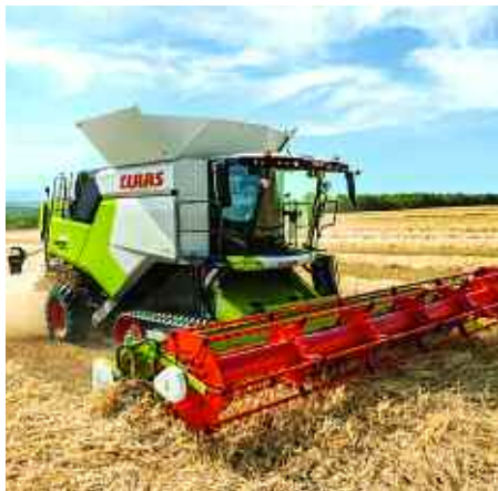
In the guts of the Trion series is an 8.9 or 6.7 litre Cummins six-cylinder Stage V engine.
