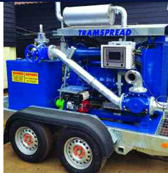
The Teletram 2020 GSM remote control can be connected via a smartphone.
