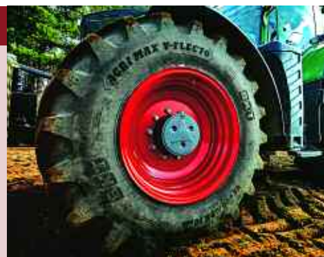
The V-Flecto tyre combines high performance in a wide-footprint tyre at low inflation pressure, bringing soil compaction benefits.
