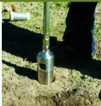
Soil cores were taken to a depth of 30cm from a sandy soil in Poland using a Van der Horst sampler.
