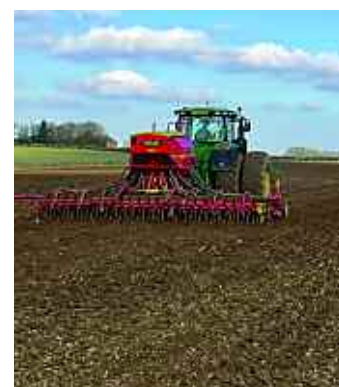
Alex has a FieldView Drive fitted to his drill which enables him to vary the seed rate across the field.
